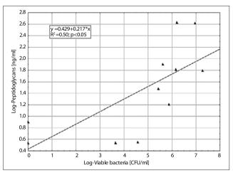
Figure 1. Relationship between the number of viable bacteria and peptidoglycans in examined cutting fluids
